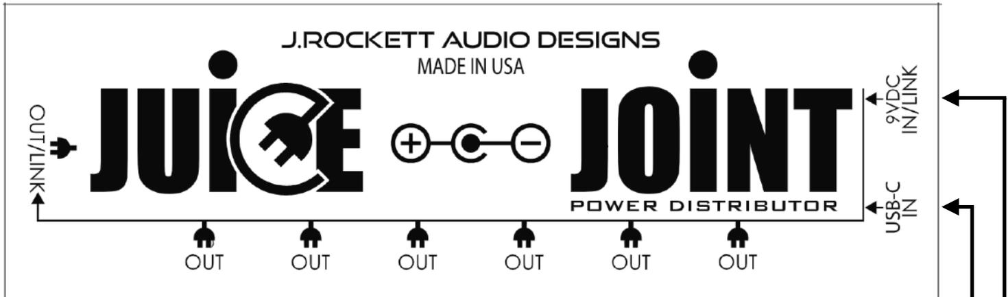
**USB-c INPUT** - This input is designed to take a typical mobile device charger rated at 5V only. **Please do not use anything other than a 5V charger.** All 5V chargers are internally converted to 9V inside of the JUICE JOINT. Wattage is not a concern so you can use larger wattage chargers as long as they are 5V. The MAX amperage that the Juice Joint input can take is 2 Amps, please do not exceed 2 Amps on either input.
