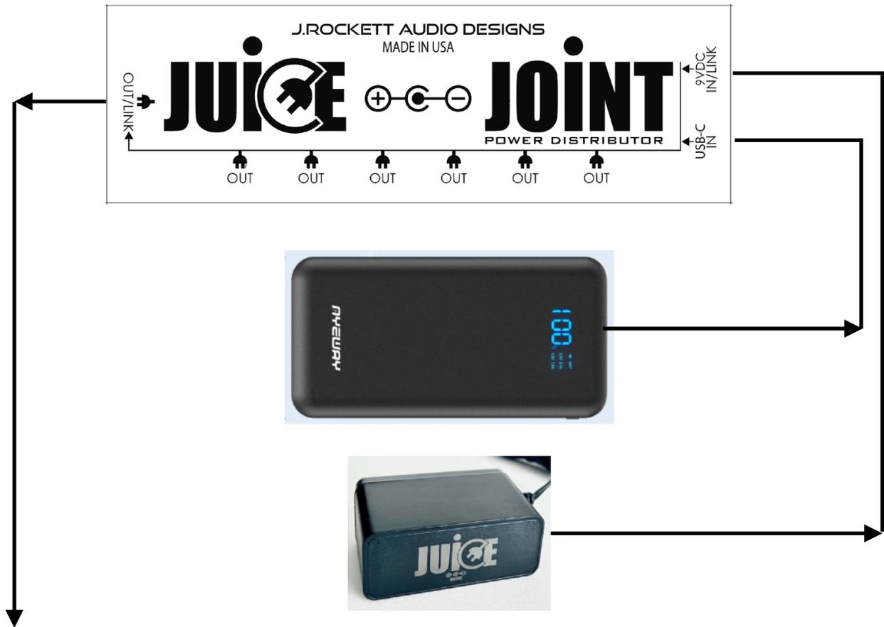
The Battery and our JUICE POWER SUPPLY can power the JUICE JOINT or the JUICE BAR depending on which you own. If you own both you only have to power the JUICE BAR. The JUICE JOINT gets its power from the JUICE BAR.
